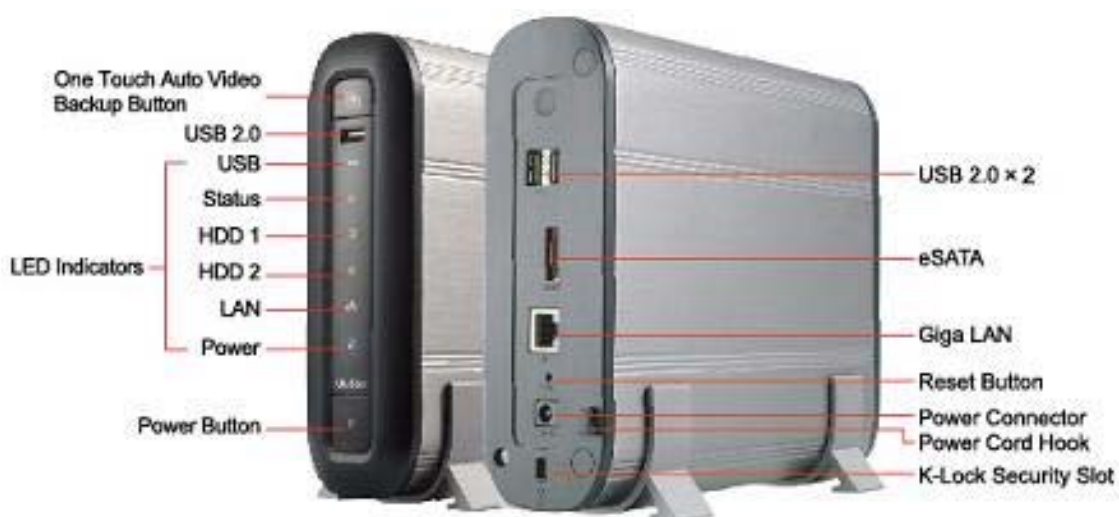
Rys.51 Serwer Q-nap Vio-Stor-101; rejestrator NVR (Network Video Recorder) oparty na systemie Linux .
